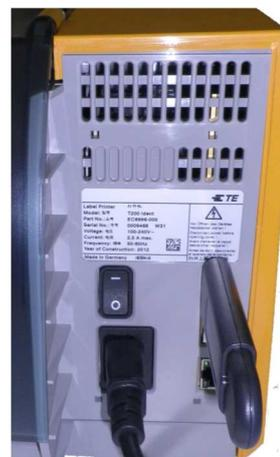
Figure 2 - USB WLAN dongle fitted
