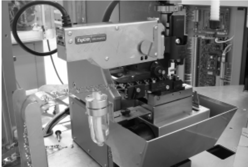
Non-Adjust System III Applicator (No Wire Crimp Height Adjustment)
