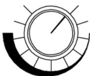
The Speed Control Knob determines the machine speed (active in both normal operation and Jog operation) Speed increases as the knob is turned **CLOCKWISE**.
