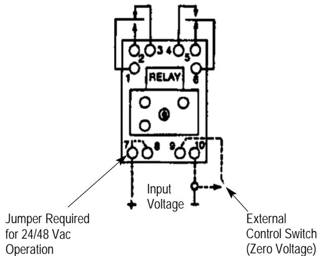
Note: External Wiring Shown by Broken Lines
