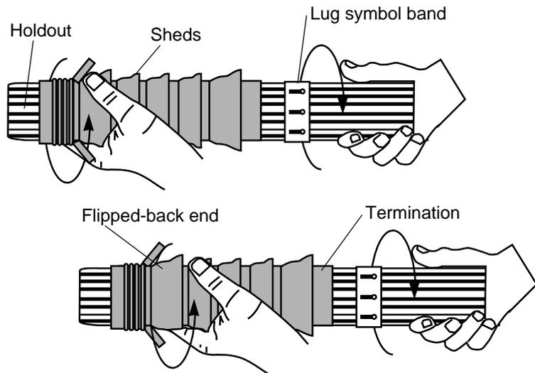
Hold the termination in one hand and the holdout in the other. Gripping firmly, twist the termination and holdout in opposite directions. Repeat twisting the termination and holdout, moving the hand in short increments up the termination until the entire termination is felt to move on the holdout.
