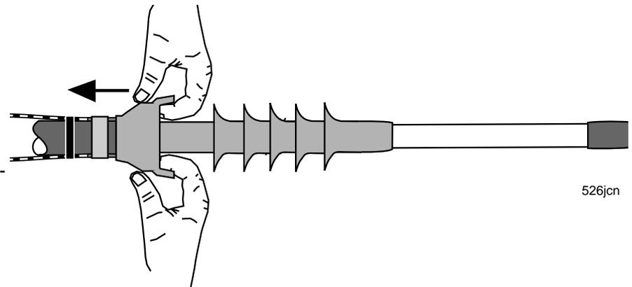
After installation, gently slide the termination so that the end aligns with the edge of the marker tape installed in step 6. Make sure the termination length is in accordance with the dimensions shown.
