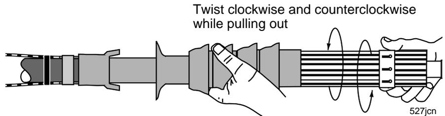
Using the pull tabs, pull the flip-back portion away from the main termination, at the same time working the first two fingers of each hand between the flip-back and main termination. Pull the stretched out flip-back over the cable jacket and sealant.
