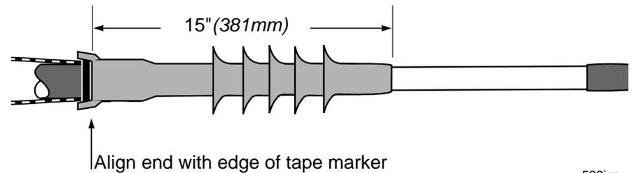
Having positioned the termination, now wrap one layer of tape sealant over the end of the termination and 1/4" (6mm) onto the cable insulation as shown.
