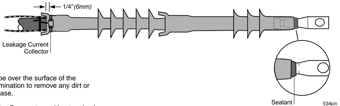
Wipe over the surface of the termination to remove any dirt or grease.
