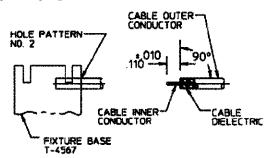
2.0 SHAPE INNER CONDUCTOR OF CABLE 2.1 TRIM INNER CONDUCTOR TO LENGTH
