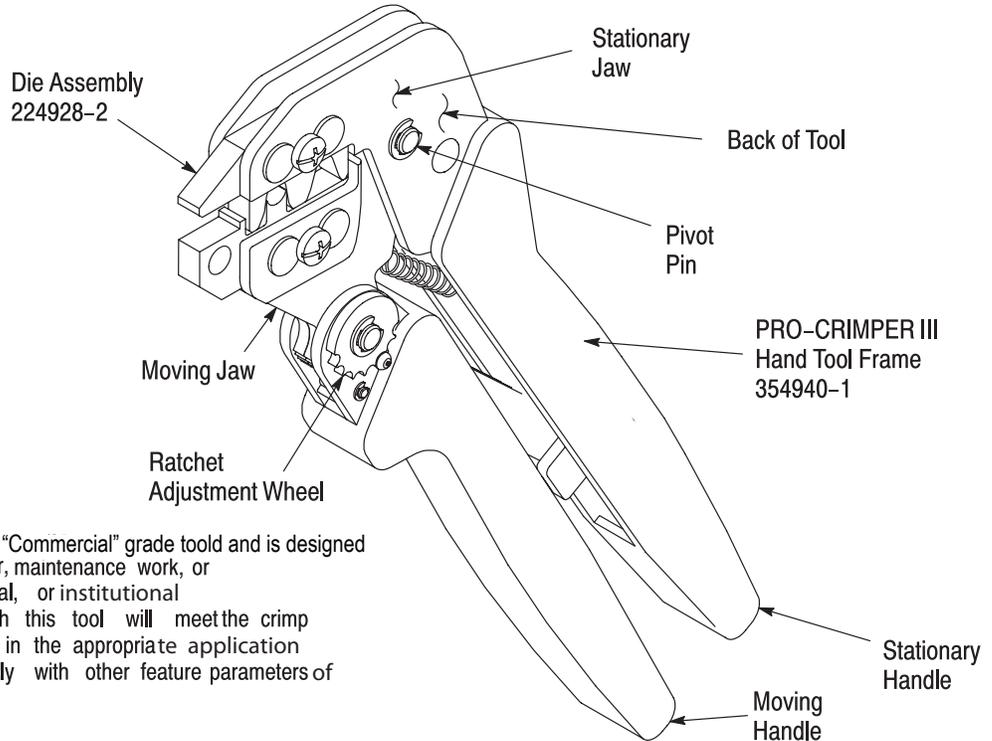
The PRO-CRIMPER Hand Tool is a "Commercial" grade tool and is designed primarily for field installation, repair, maintenance work, or prototyping in industrial, commercial, or institutional applications. Product crimped with this tool will meet the crimp height requirement for handtools in the appropriate application specification but may not comply with other feature parameters of the specification.
