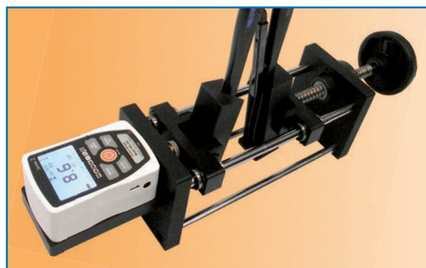
Handle force, measured at the factory, is a critical component of precise, reliable crimping.
