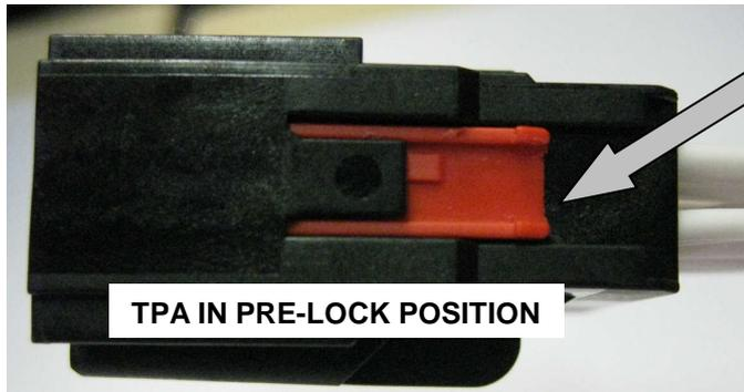
DELIVERY CONDITION OF THE MALE CONNECTOR WITH THE FRONT LOADED TPA (SPACER) IN PRESET POSITION. THE FRONT LOADED TPA (SPACER) IS ELEVATED.
