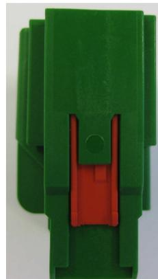
Insert tool to unlock contact
