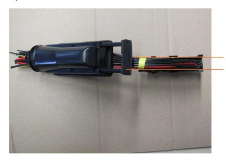
Check that's the cables are inside the two orange lines.
