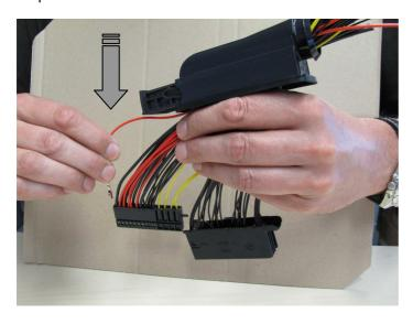
Insert crimped terminals into the housings: MQS FEMALE HOUSING; 22POS. MIXED FEMALE HOUSING; 26POS.
