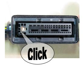
Push the housing into the cover and move it to the end lock position.
