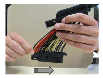
Insert MQS FEMALE HOUSING; 22POS. and MIXED FEMALE HOUSING; 26POS. In to COVER; FEMALE HOUSING 48POS.
