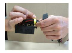
Fix the cables with a tape
