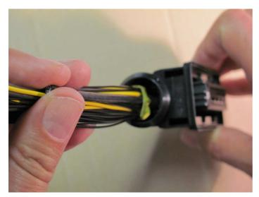
Check that's the tape is not in the cable tie area.
