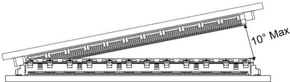
2. Then pull the Receptacle the other side upwards.
