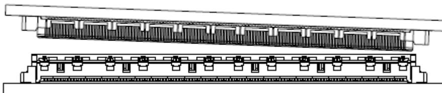
3. Separate the Receptacle and Plug using slight pressure completely.
