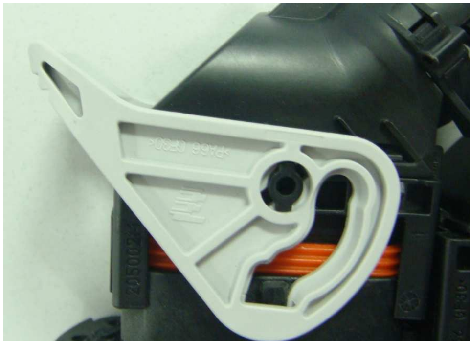
Figure 18 (incorrect pre-insertion, 不正确的预插状态)
