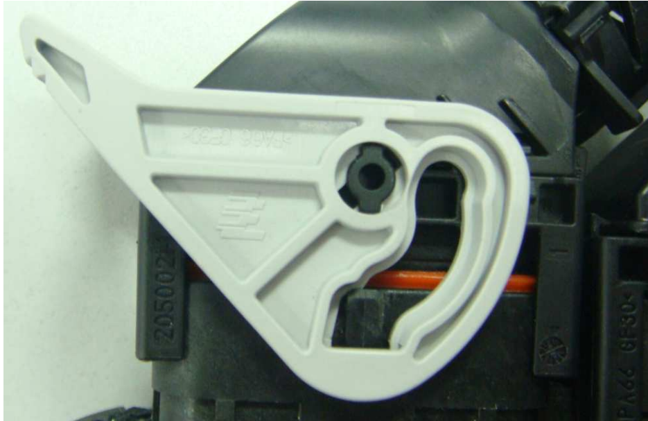
Figure 17 (Correct pre-insertion, 正确的预插状态)
