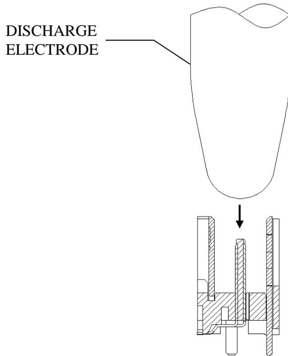
Fig.2 Test method of Electrostatic Discharge
