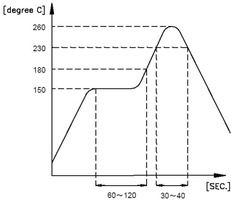
Fig.3 Temperature Profile of Reflow Soldering
