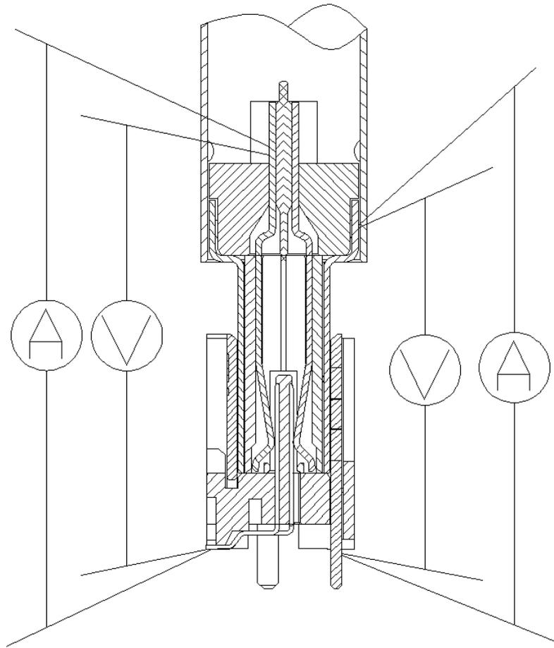
Fig.1 Contact and Shell Resistance Measuring point
