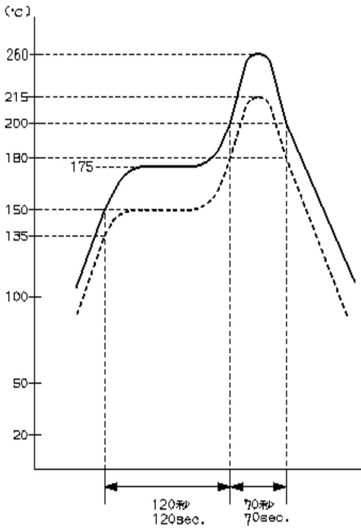
Fig. 3 Reflow Condition
