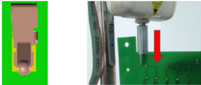
Fig. 5: Test Condition for Peel off strength (Long pad direction)
