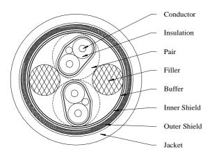
Note: Drain wire orientation (relative to outside of cable) will vary due to pair twisting.
