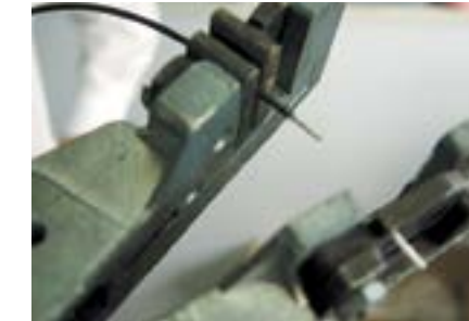
Wire stripping with a recommended tool will allow the insulation to be removed accurately without damaging the wires.
