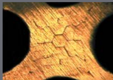
A good crimp showing the individual wires compressed evenly.
