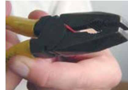
Not the best way to strip insulation. Pliers may remove the insulation, but are also likely to break and remove strands of the wire too.
