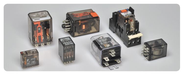
The robust designs of panel plug-in relays make them a popular choice for many different industrial and commercial applications. Socket mounted relays are often used in applications where many operations are expected, and the operational life of the equipment is likely to exceed the operational life of the relay. Elevator/escalator controls, commercial HVAC, and street lighting are a few such applications.
