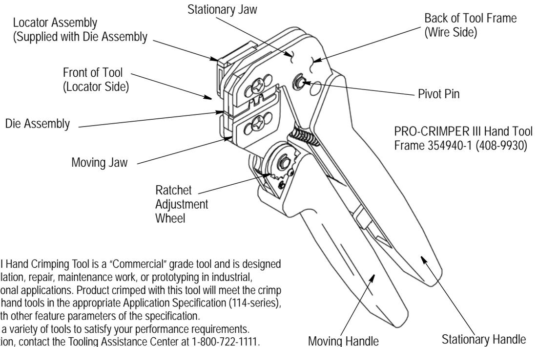
The PRO-CRIMPER III Hand Crimping Tool is a "Commercial" grade tool and is designed primarily for field installation, repair, maintenance work, or prototyping in industrial, commercial, or institutional applications. Product crimped with this tool will meet the crimp height requirement for hand tools in the appropriate Application Specification (114-series), but may not comply with other feature parameters of the specification.
