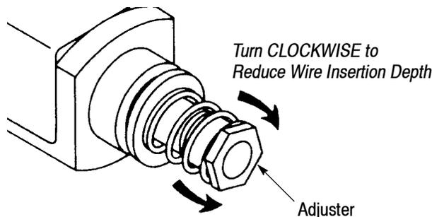
Turn **COUNTERCLOCKWISE** to Increase Wire Insertion Depth
