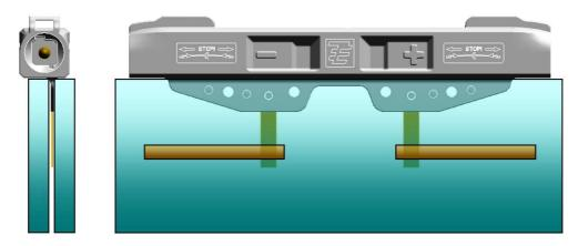
Fig. 3: Edge Connector with glass plates
