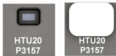
Laser marking on HTU20P(F) sensor
