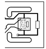
Example of HTU21D(F) sensor mounting with slits mills to minimize heat transfer
