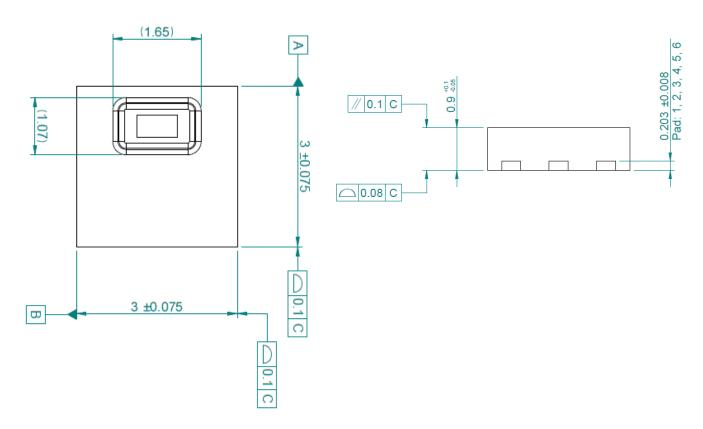
Dimensions are given in mm, tolerances are ±0.1mm. The die pad (thermal center pad) is internally connected to GND.
