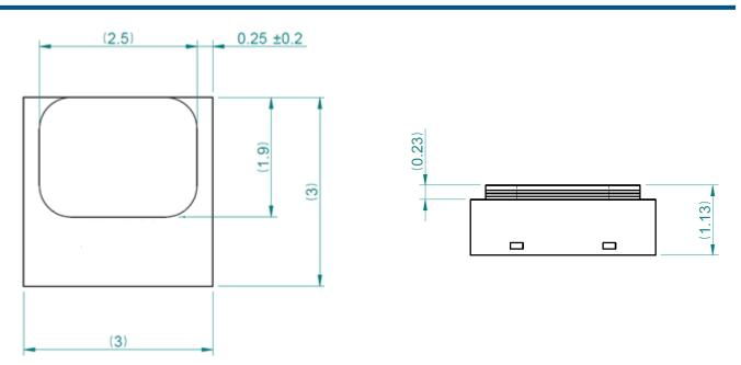
Dimensions are given in mm, tolerances are ±0.1mm. The die pad (thermal center pad) is internally connected to GND.
