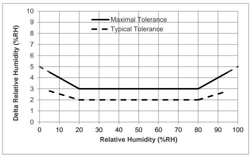
• HTU21D(F) sensors are specified for optimum accuracy measurements within 5 to 95%RH.
