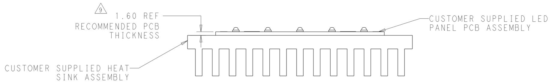
9 APPLICATION NOTE: IN ADDITION TO USE WITH COB LEDS THE SCALABLE LED HOLDER CAN BE UTILIZED TO MAKE AN ELECTRICAL CONNECTION TO FR4 OR IMS PCB ASSEMBLIES. RECOMMENDED DIMENSIONAL INFORMATION FOR THIS TYPE OF APPLICATION IS SHOWN IN THE DRAWING VIEWS ABOVE.
